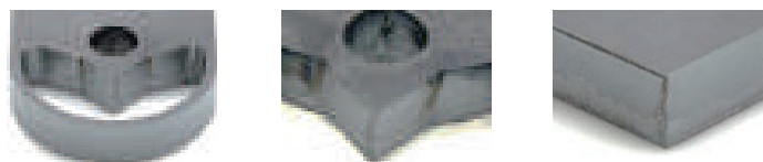
Bevel reduction and sharp corner detail (LBC technology + Smart edge)
