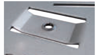
Downward bridge forming
